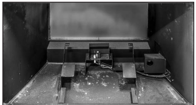
Figure 40: The rear liner can now be removed. Use a vacuum to clean up the bare firebox if needed.
