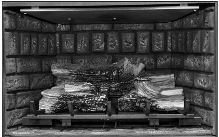
Figure 42: Place both the left and right mid logs in the middle of the air deflector. Make sure the bottom holes align with the pins in the air deflector.
