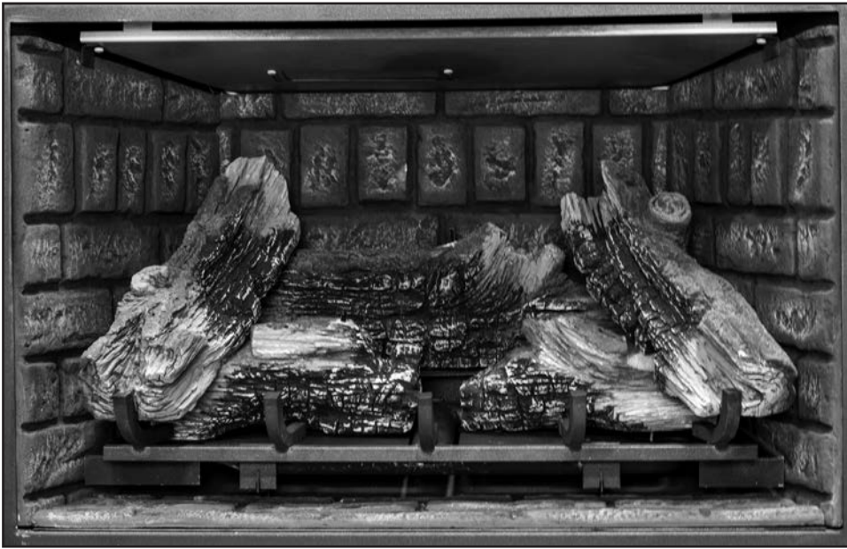
Figure 44: Install the right top log on top of rear log and right mid log. Locate the bottom on the far right grate arm.
